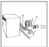
1. Leave an opening in the wall to the left of the dryers proposed position.
